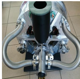
Figure 5: HTS motor of RESUM project.
