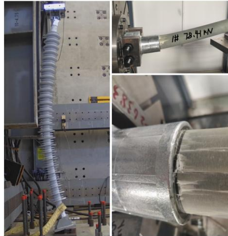
Figure 3 : Line post insulator failure modes under compression buckling (left) and bending stresses with FRP core damage (right)
