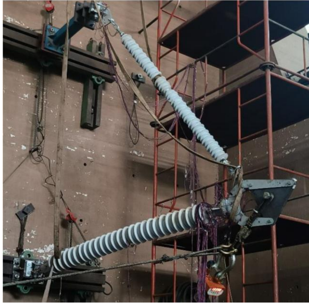
Figure 9 : Full-scale combined load testing of braced assembly with 110 mm diameter post insulator.
